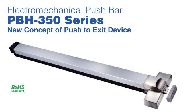
The PBH-350 Series Electromechanical Push Bar is designed for use on emergency exit doors. It provides a convenient means of escape by simply pushing on a horizontal bar fitted across the width of a door. It also features preload release capability that overcomes door preload problems, such as air-conditioning pressure, changes in the weather, warped doors or doors with weather stripping.
